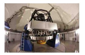
2.5m diameter; 3sq.deg. FoV Telescope accepted on 5th Feb 2016.
