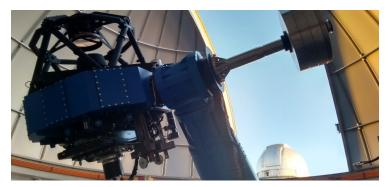
80cm diameter; 2sq.deg. FoV T80Cam:  $9k \times 9k$  CCD; 0.553''/px
