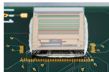
Wire-bonding of the ASIC control pads
